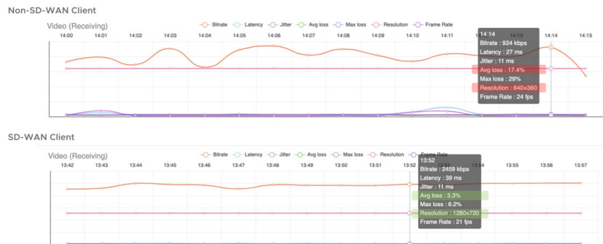
FIGURE 3: VMware SD-WAN: loss mitigation for better resolution for Zoom video communications
